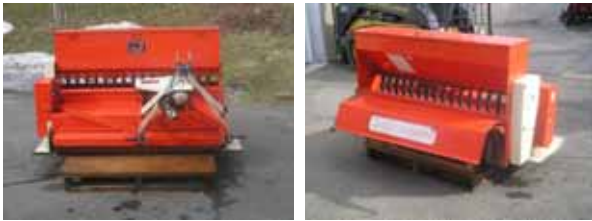
Jacobsen seeder, 3 pt. hitch, tractor mount;
