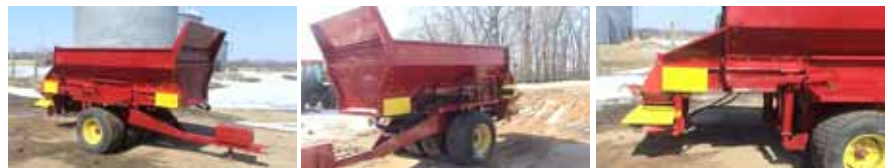
2004 Tye Crop top dresser with spinners & belt conveyor
