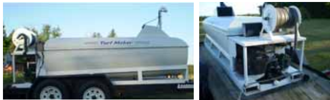
Turfmaker 700 Hydro-Seeder, 18 hp Kohler Command engine, mechanical agitation, 700 gal. tank, covers 5000 sq. ft. per load, 275 ft. of hoses, 3 applicator nozzles, approx. 6 yrs. Old, good condition, trailer not included.
