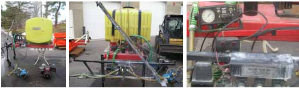
Toro Workman 200 gal. mounted sprayer, pto, Tee Jet spraying system, 3 electrical solenoids;
