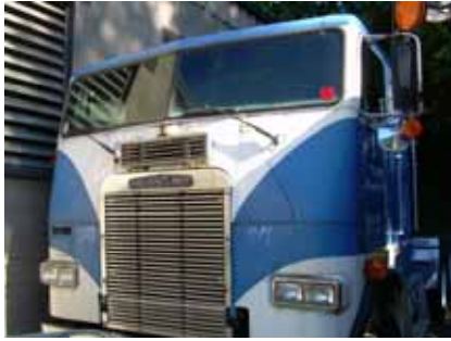
1989 Freightliner , cab over, 12,000 lb. front, 40,000 lb. rear, standard hook ups
