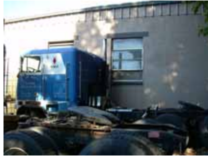
1989 Freightliner , cab over, 12,000 lb. front, 40,000 lb. rear, standard hook ups
