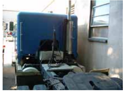
1989 Freightliner , cab over, 12,000 lb. front, 40,000 lb. rear, standard hook ups
